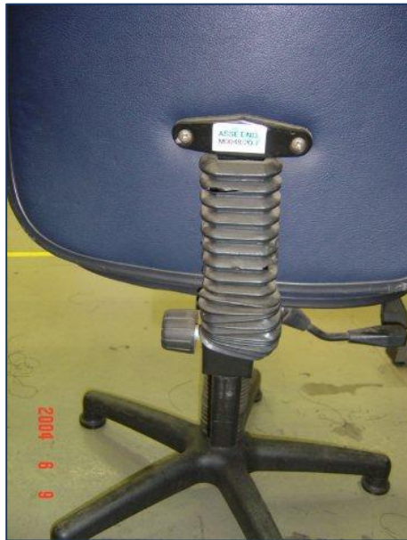
Picture 3.9 Height adjustable back rest of a sewing-machine operator's chair
