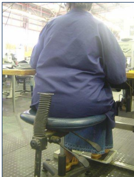
Picture 3.10 A broken back rest
