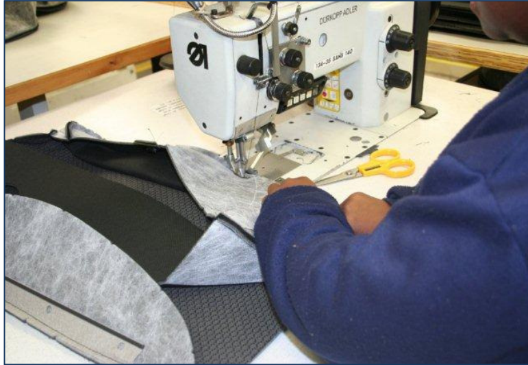
Picture 3.2 Straight stitching of bulkier parts
