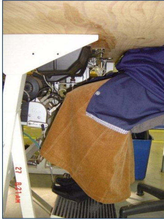
Picture 3.21 A sewing-machine operator working in a seated work station with sufficient leg space underneath the sewing table.
