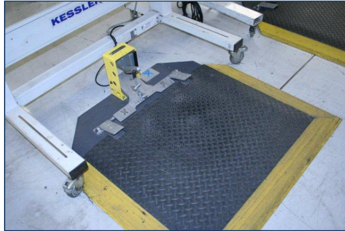
Picture 3.13 Shock-absorbing carpets for the stand-up work stations
