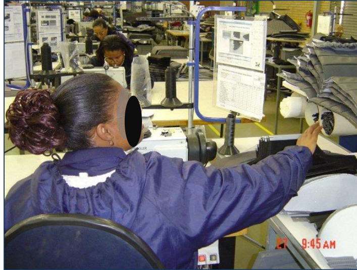
Picture 3.3 The seated work station demonstrates storage heights
