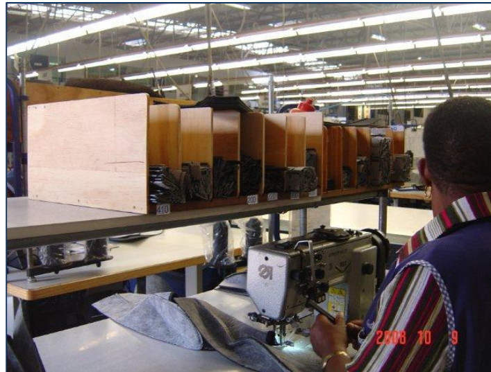
Picture 3.4 The stand-up work station demonstrates storage heights
